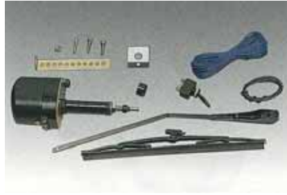
LMWT-340 FOR REAR WIPER MOTOR 12V/24V
